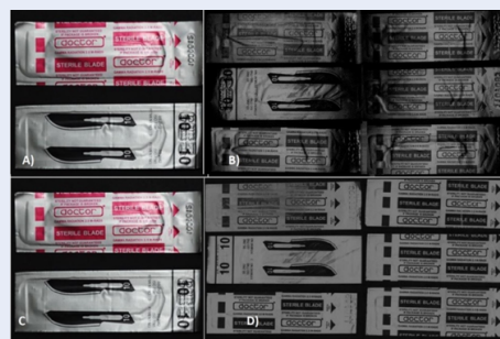
Figure 2: Image of the aluminum foil package containing a disposable surgical scalpel captured by: Smartphone camera with ambient light source (A and C), Mono camera with coaxial lighting technique (B), and Dome lighting (D)
